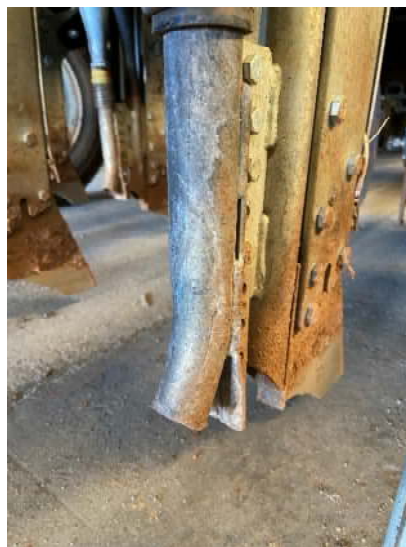
Knife point on Kalyx cone seeder, press wheels and diffusers optimising seed and fertiliser placement for the Incitec Pivot Fertilisers Split P trials.
