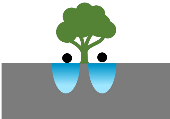
Figure 3: Representation of wetted area and root activity (blue area) for drip irrigation
